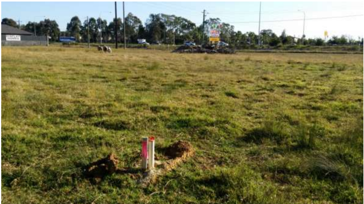
Groundwater monitoring well at the western portion of the site.
